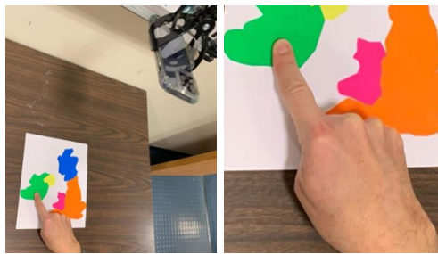
Fig. 2. Left: Experimental setup shows iPhone 14 Pro mounted above the British Isles tactile map in cellphone holder with the user making a pointing gesture on the map. Right: close-up of pointing gesture. The five levels of text labels for the region being pointed to are: “Republic of Ireland”; “2: Capital is Dublin”; “3: Population 4.9 million”, “4: Area 27133 square miles”, “5: Limerick is another city in Ireland”.
